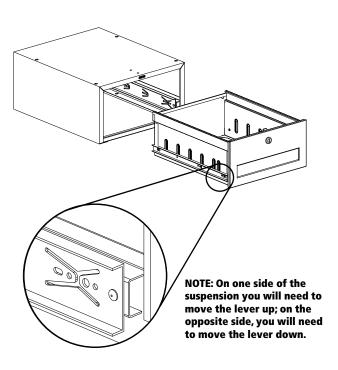
2. Attach the two mounting brackets (Ref. No. 1) in the desired location on the workbench top. It is most common to place the drawer to either the far left or far right side of the bench, but can be placed anywhere that there are two holes in the bench top that are 15" apart. Secure with two 1/4"-20 x 5/8" bolts (Ref. No. 5) per mounting bracket.
