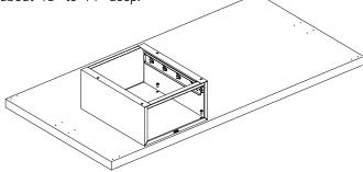
**3.** Secure the housing to the top, using four #14-3/4" hex head slotted wood screws (Ref. No. 7).
