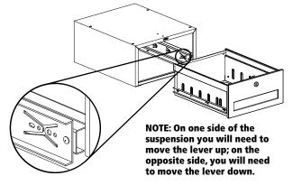
**2.** Bolt housing together with four <sup>1</sup>/4"-20 bolts and nuts (Ref. No's 5 & 6).
